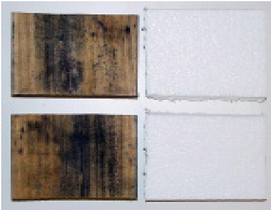
Southern Yellow Pine with Mold Growth
