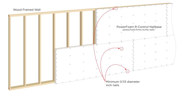
**Notice:** PowerFoam R-Control insulation contains a flame retardant; however, it should be considered combustible and should not be exposed to sources of ignition. The product will ignite when exposed to open flame or welding torches.
