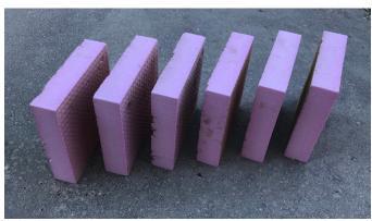
The samples were tested following the industry standard for R-value, ASTM C518, at a mean temperature of 75°F.
