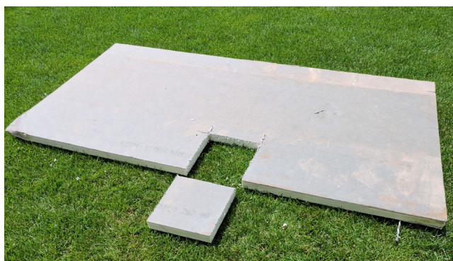
Figure 5. 17 year old polyiso sample
