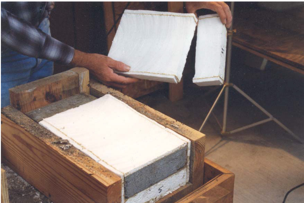
#64 TEST FIXTURE - cut open to reveal limited termite damage.
