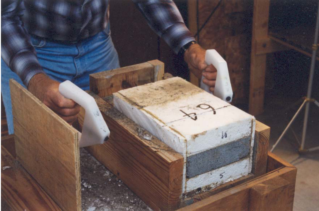
#64 TEST FIXTURE - Examination of PowerFoam with Perform Guard after 3 years exposure. Highland site, Mississippi.
