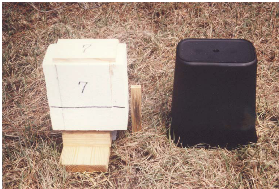
TEST FIXTURE - Prior to installation showing underground baitwood base to attract termites to site. Canister cover to protect termite activity.
